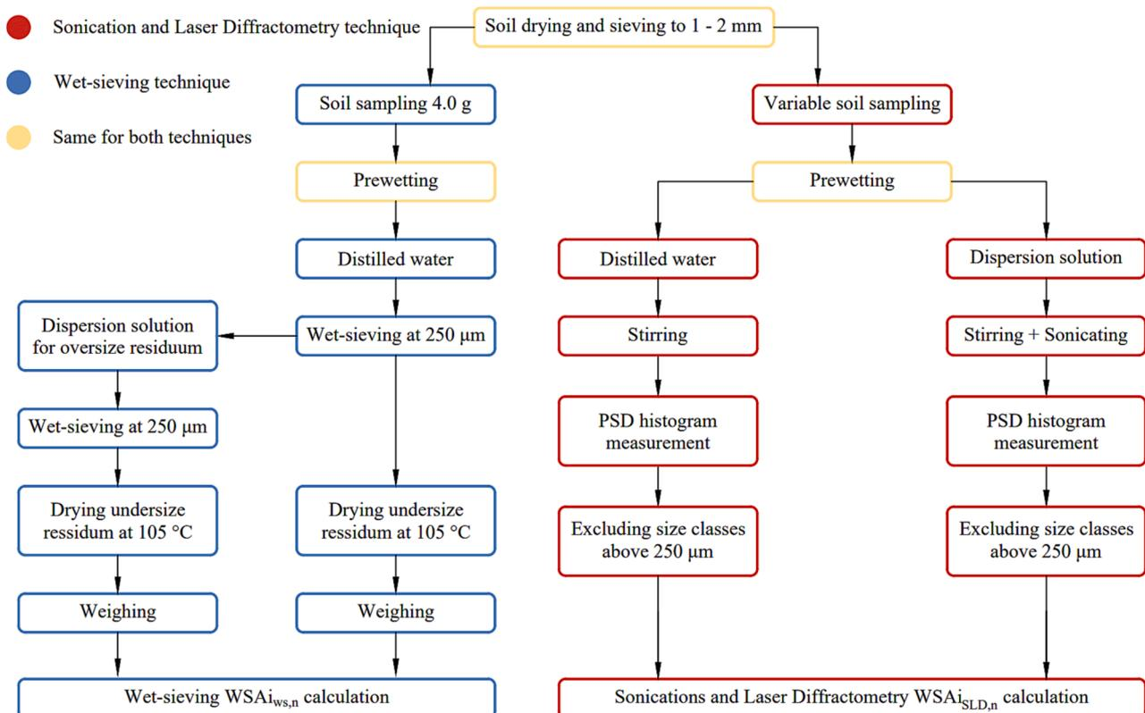
Fig. 2. Aggregate stability flow chart, simultaneous determination of WSAi by Wet-sieving and by the Sonication and Laser Diffraction approaches.
