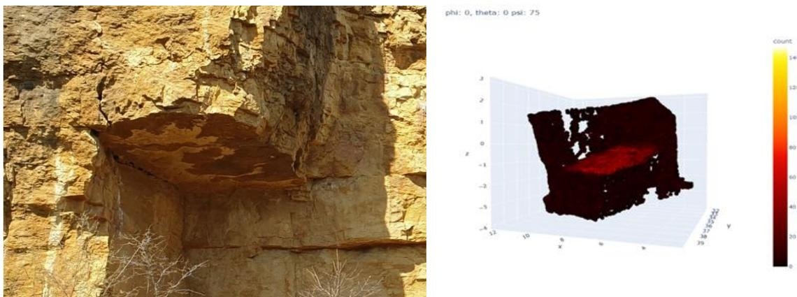
*Figure 2: on the left picture of the real data scan of the yellow quarry Ferreyres. On the right density map of the yellow quarry in Ferreyres, generated using a specific viewpoint (angle of the viewpoint =  $\phi$ : 0,  $\theta$ : 0,  $\psi$ : 75). The color range indicates the point cloud density for this viewpoint.*
