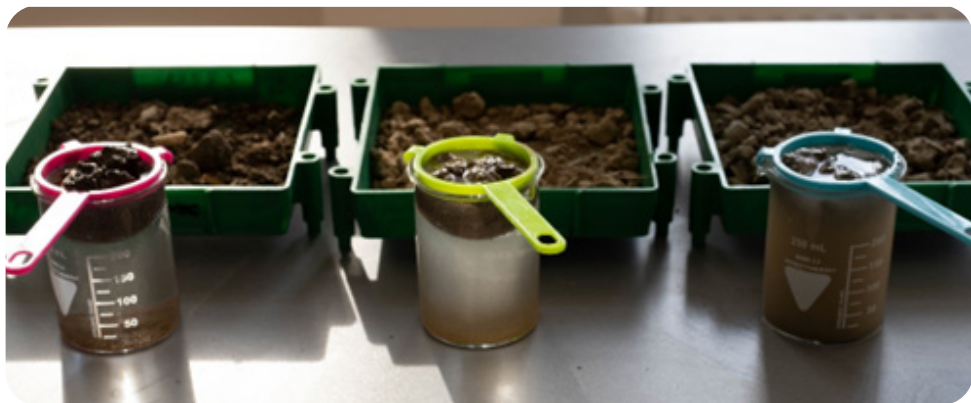
4. Abra: Results of soil aggregate stability test (see the TUDi DST app), applying tea strainer, glass and water. The stability of the soil structure decreases from left to right.
